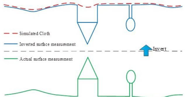
Fig. 4. Overview of the cloth simulation algorithm (Zhang et al. 2016)
